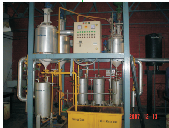
Figure 2. Biodiesel Pilot Plant at Engine Research Laboratory, IIT Kanpur
