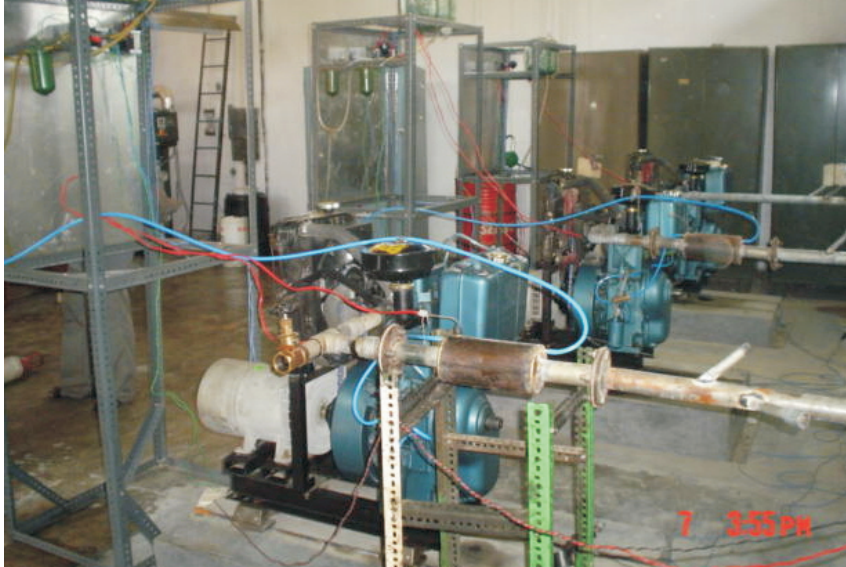
Figure 3. Engines fuelled with Straight Vegetable Oil (SVO) at ERL, IIT Kanpur
